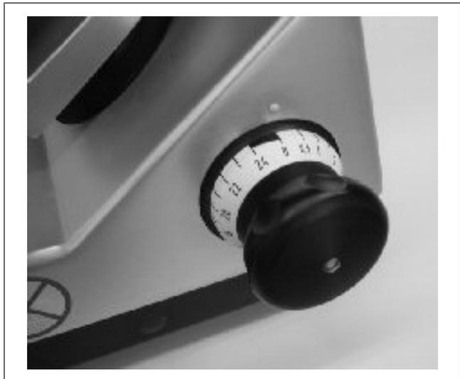
Fig. 71: Slice thickness below "0"
