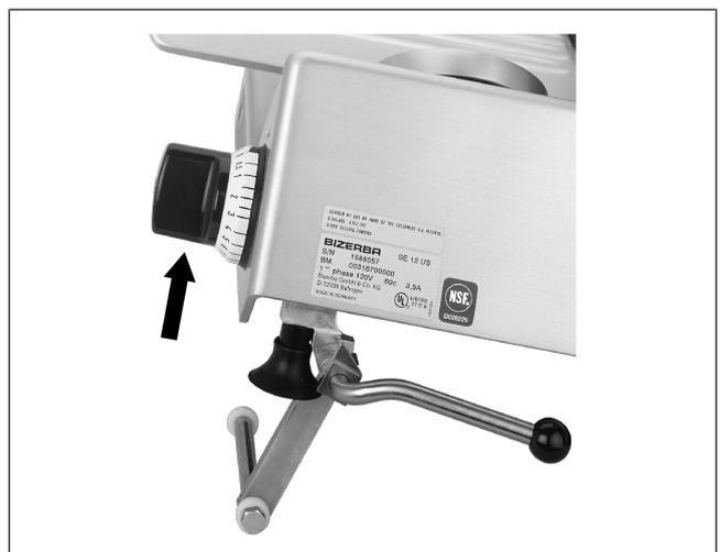
Fig. 30: Lifting device GSP H
