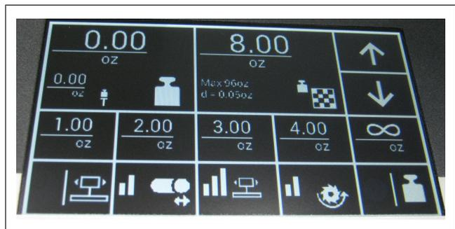
Fig. 54: Automatic operation to target weight
